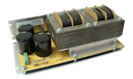
The PSA80V4A-1 power supply has a single 80V output, a voltage input of 115 or 220VAC, and power capabilities of up to 320 watts. With an unregulated output and a size of 8.30" x 4.25" x 2.81" and dual mounting position "L Bracket," the PSA80V4A-1 can be mounted just about anywhere. The PKG-342-MBC08-PS-CBL includes two wires for powering the MBC12101.
